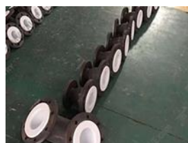
Inspection For PTFE Lining Fittings
