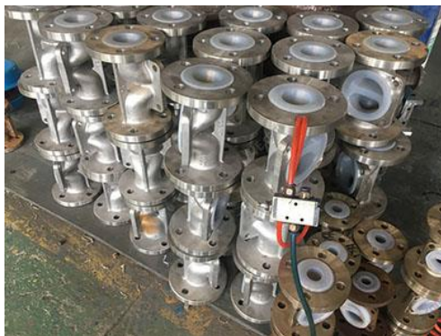
PFA Fluoropolymer Liner Of The Diaphragm Valve
